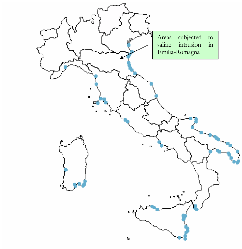
Figure 19. Areas with saline intrusion phenomenon in Italy (source: Enea 1998)
