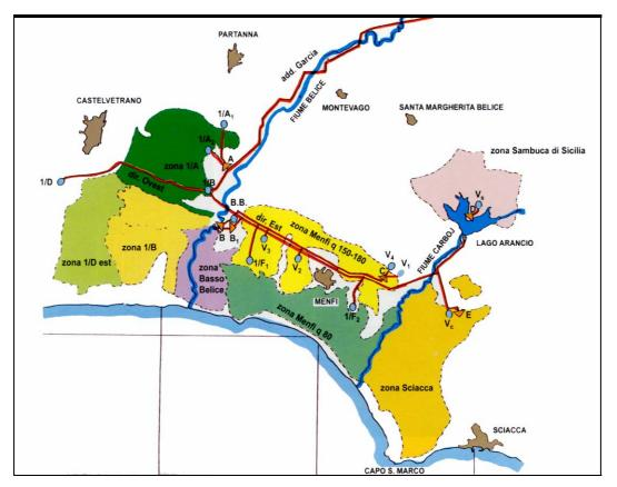
Figure 21. The hydraulic scheme of Garcia-Arancio-Belice
