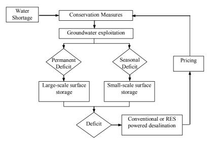
Figure 1. Potential solutions in water supply development
